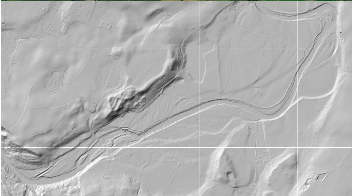
Fig 6. Digital terrain model derived from LiDAR data of the Ure flowing from bottom left to top right with the shadow intensity especially to the LB (northern) emphasising how incised the straightened extant channel has become. Paleochannels, ghosts of the channel's position over time, are evident meandering across the full width of the floodplain.
